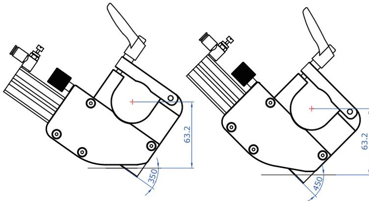
Blade angle could be varied within the range of 35 ~ 45° keeping the same gap to the web surface
