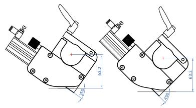
Blade angle could be varied within the range of 35  $\sim$  45° keeping the same gap to the web surface
